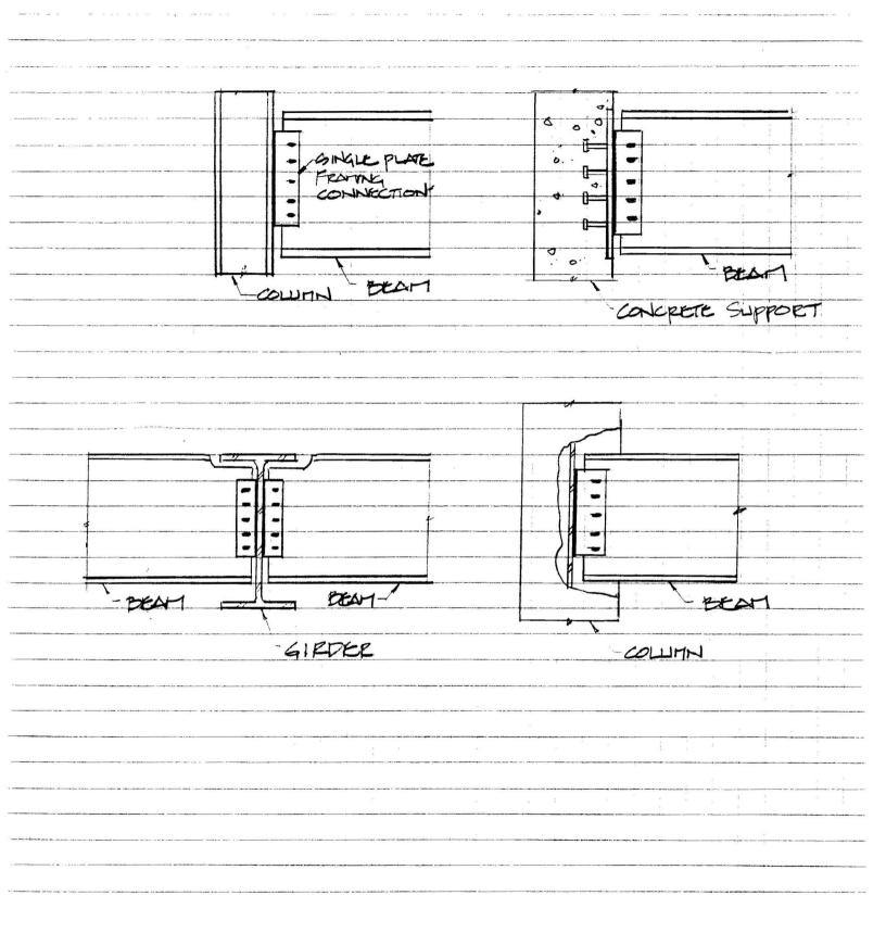
Figure 1-1: Typical applications of single plate framing connections
