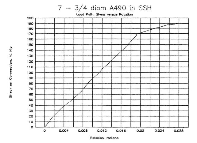
Figure A-3: Load path for 7-bolt specimen
