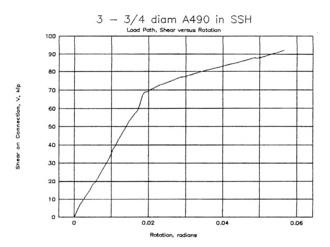
Figure A-1: Load path for 3-bolt specimen
