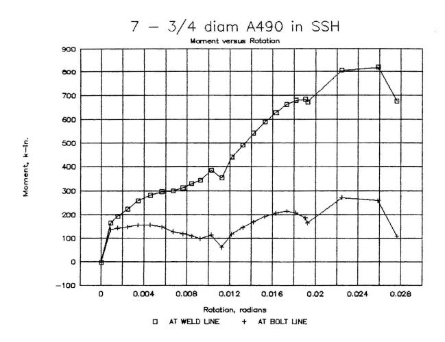
Figure 4-3: Moment-rotation behavior of 7-bolt specimen
