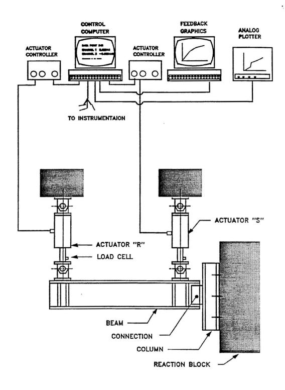
FIGURE 2-7: TEST SET-UP USED IN THE INVESTIGATION
