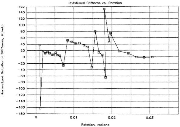
Figure 4-8: Rotational stiffness behavior of 9-bolt specimen
