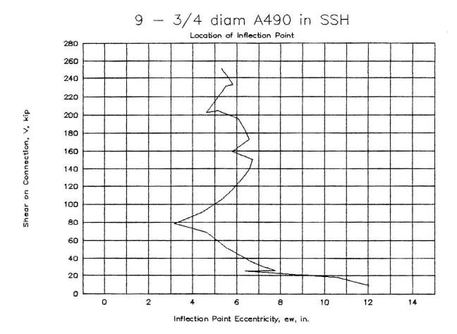
Figure 4-12: Reaction eccentricity behavior of 9-bolt specimen
