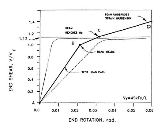
FIGURE 2-6: SHEAR-ROTATION CURVE USED FOR THIS PROJECT
