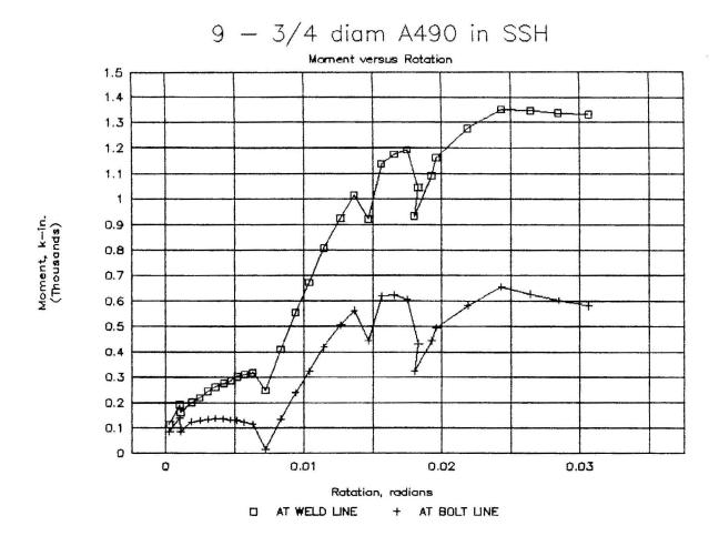
Figure 4-4: Moment-rotation behavior of 9-bolt specimen
