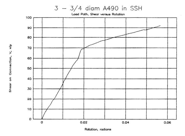
Figure A-1: Load path for 3-bolt specimen
