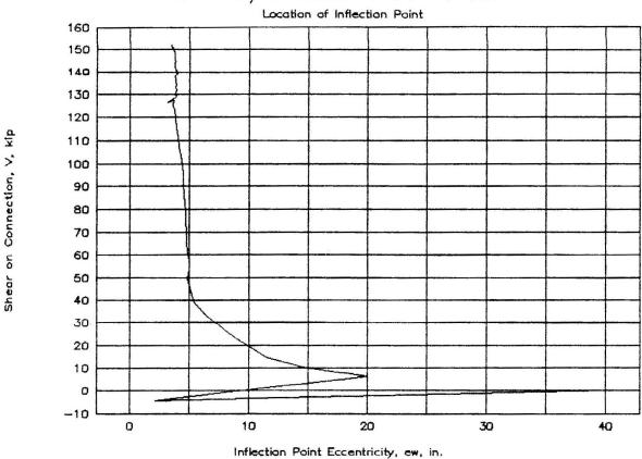
Figure 4-10: Reaction eccentricity behavior of 5-bolt specimen
