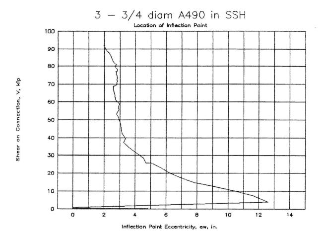
Figure 4-9: Reaction eccentricity behavior of 3-bolt specimen
