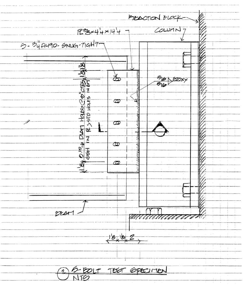
Figure 2-2: Five-bolt test specimen
