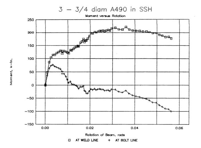
Figure 4-1: Moment-rotation behavior of 3-bolt specimen
