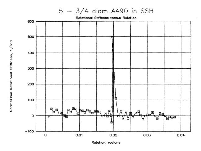
Figure 4-6: Rotational stiffness behavior of 5-bolt specimen
