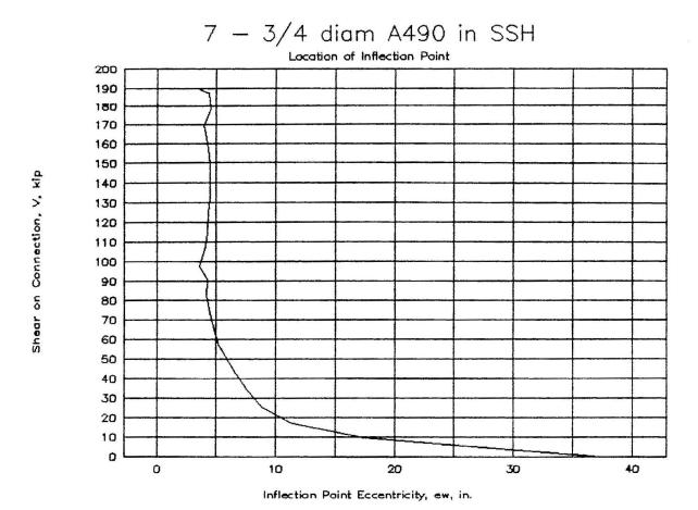
Figure 4-11: Reaction eccentricity behavior of 7-bolt specimen
