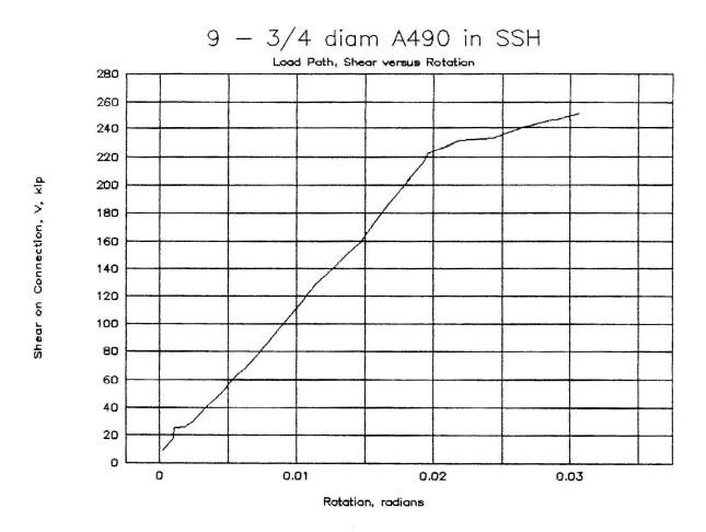
Figure A-4: Load path for 9-bolt specimen
