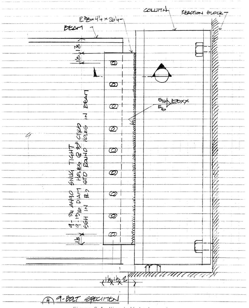
Figure 2-4: Nine-bolt test specimen
