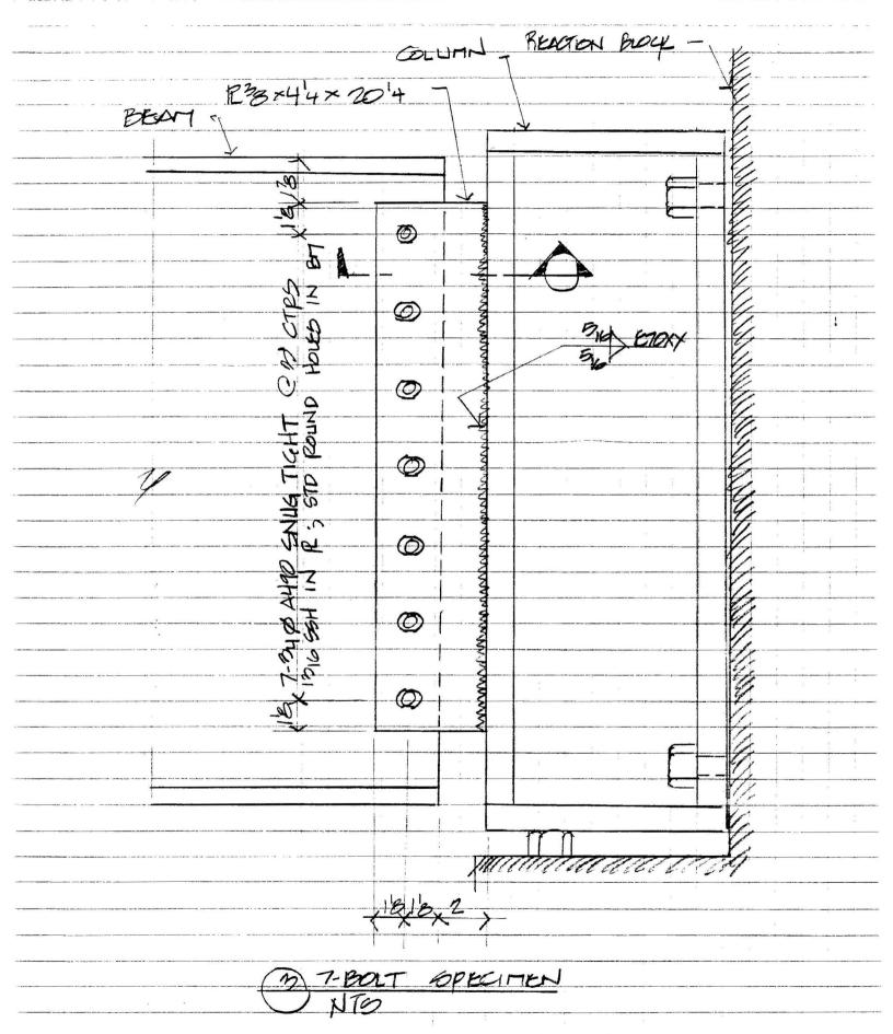
Figure 2-3: Seven-bolt test specimen
