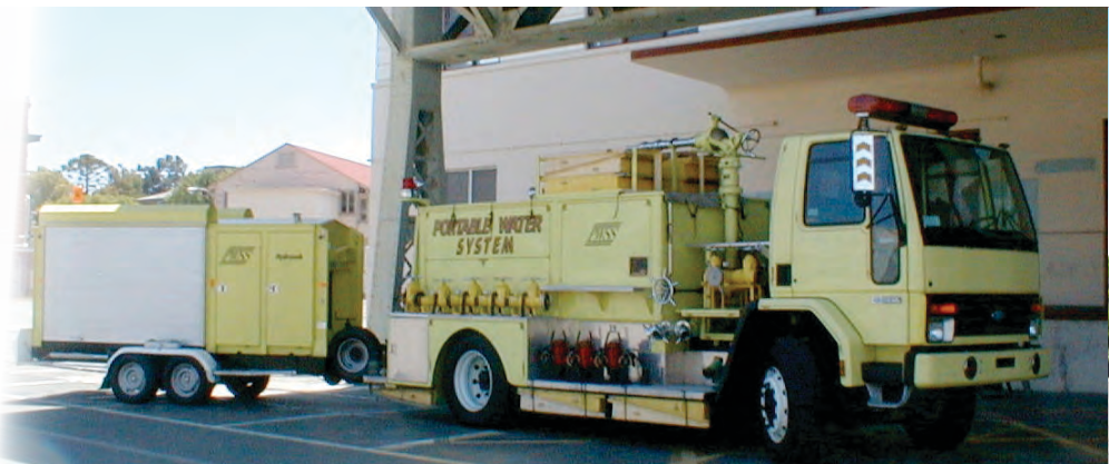
Portable Water Supply System (PWSS), Vallejo FD; Source: Scawthorn
